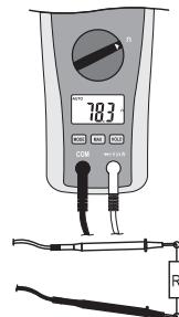
→ If you carry out a resistance measurement, make sure that the measuring points which you contact with the test prods are free from dirt, oil, solderable lacquer or the like. An incorrect measurement may result under such circumstances.
