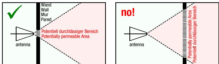
For the definition and installation of shielding measures as well as surveying their effect, professional advice is recommendable. Anyway, the area covered by shielding material should be much larger than the leak itself.
