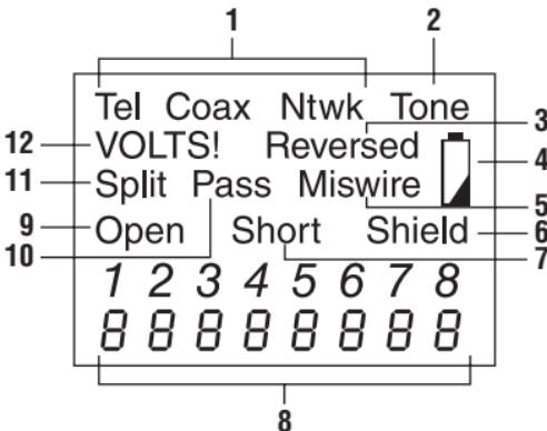
\* The NETcat Micro requires one 9 V snap-type battery (alkaline types are recommended). When the low battery icon is displayed, a few hours of typical use remain. Using the unit with a low battery will eventually affect the accuracy of measurements.
