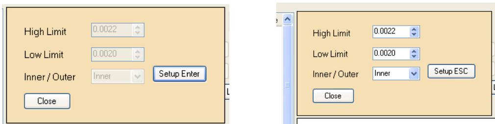
**Setup Enter** : When button is pressed, the upper/lower limit and the mode can be modified; when button is up, the settings will be sent and saved in the device.
