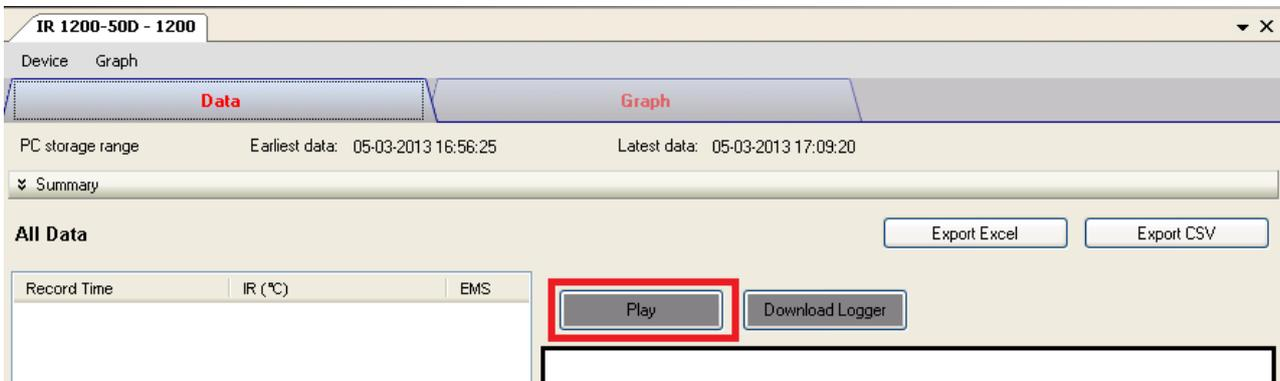
In real time mode, pressing the trigger on the device will start sending data to PC, no data will be sent if the trigger is not pressed.
